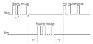
However, these parameters take on particular importance in the setting up of a network made up of a large number of instruments, in fact if T2 and T3 are not restricted by determined maximum values, the time needed by the master (PC) to interrogate the entire rate may be excessive. It is also necessary to set the minimum values to avoid problems of conflict between different devices. The accepted values are listed inside this table:
